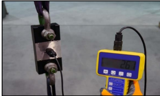
Fig. 2. NDT Load Testing
